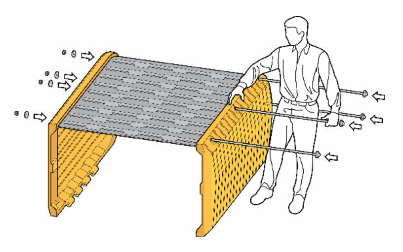
Stand the assembled sidewall and back panel upright and place the all thread rod through the 3rd hole from the bottom using the same steps to attach this rod as the previous rods.
