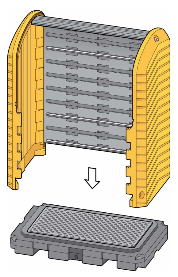
Place the assembled sidewalls and back panel on top of the spill pallet (1) with the grate (2) installed.
