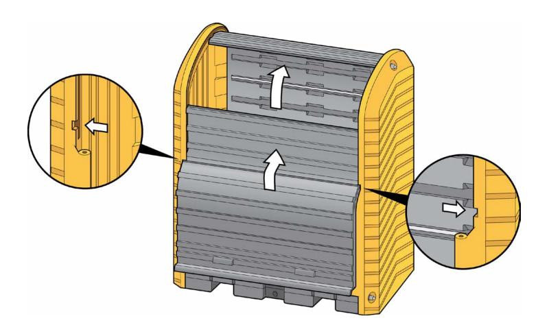
On the back panel tighten the 3rd threaded rod from the bottom to a distance of 59  $\frac{3}{4}$ " between the sidewalls. Then tighten the top threaded rod to a distance of 59  $\frac{3}{4}$ " between the sidewalls.
