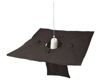
The Drain Warden operates in a similar fashion to a gross pollutant trap. Runoff water will tend to 'swirl' inside the Drain Warden when it enters the pit. Any particulate greater than the pore size of the fabric will be trapped by the geotextile fabric. The hydrocarbons will be absorbed by the hydrophobic boom suspended beneath the grate.
